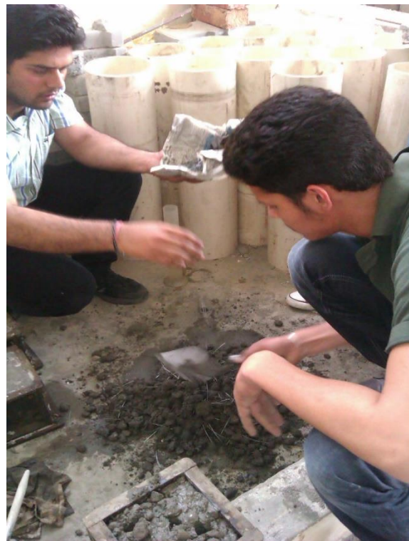
Mixing of aggregate with steel bars.
