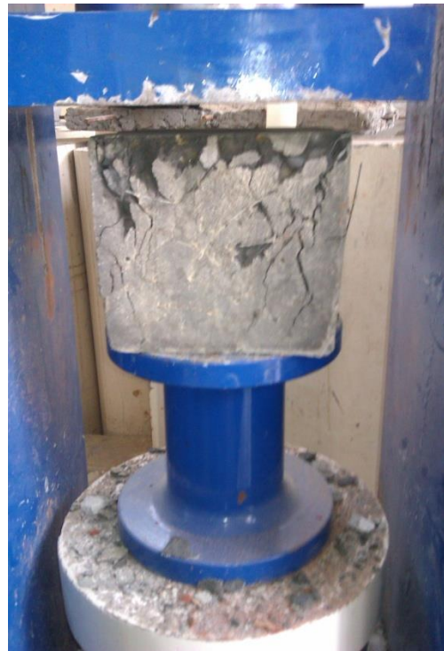
Checking of compressive strength concrete moulds having steel & iron reinforcement.
